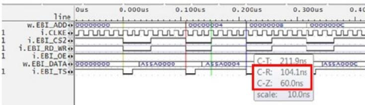
Figure 4.2 32-bit data output using EBI MRAM
