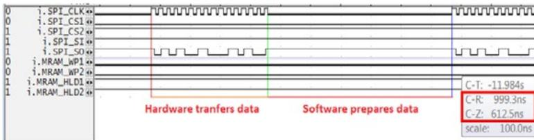
Figure 4.1 16-bit Data output using SPI MRAM
