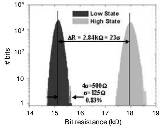
**Fig. 3:** Low- and high-state resistance distributions measured at operating bias and with series transistor resistance. Data are from a 64kb sample of a 4Mb device. (From B. N. Engel *et al.*, *IEEE Trans. Magn.* **41**, 132 (2005). © 2005 IEEE).
