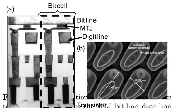
Figure 1. (a) Cross-section TEM image of a bit cell showing the bit line, MTJ, and digit line, and underlying CMOS circuitry. (b) Top-down SEM of toggle MRAM MTJ bits and their underlying bottom electrode.
