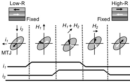
**Fig. 2:** Schematic of a toggle MRAM bit with the field sequence used to switch the free layer from one state to the other. The fields  $H_1$ ,  $H_1 + H_2$ , and  $H_2$  are produced by passing currents,  $i_1$  and  $i_2$  through the write lines. (From B. N. Engel *et al.*, *IEEE Trans. Magn.* **41**, 132 (2005). © 2005 IEEE).
